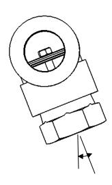
Side view of manifold showing the check valve in the open position.
